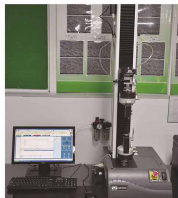
常温延伸率-抗拉强度试验机 Elongation At Room Temperature-Tensile Strength Testing Machine
