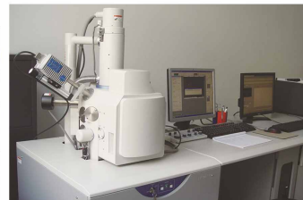
SEM即扫描电子显微镜 SEM Namely Scanning Electron Microscope
