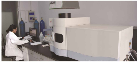
ICP (全谱直读等离子体发射光谱仪) ICP ( Full Spectrum Of Direct-reading Plasma Emission Spectrometer )
